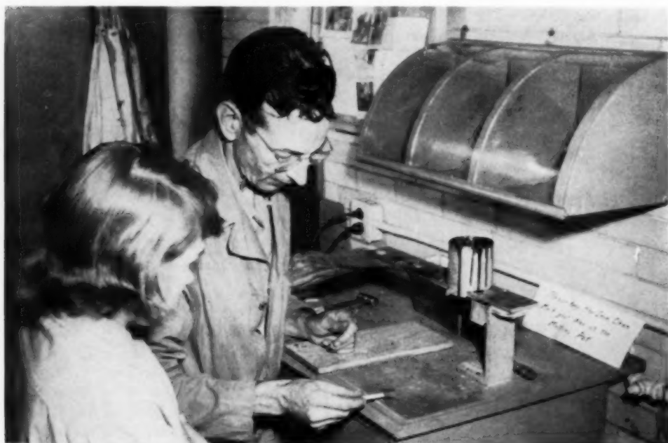
Instructor Bert Thornton demonstrates the proper technique for "Dopping" a stone to be polished to a stick so that it may be held against the grinding wheels, sanded and polished with greater ease. A special wax is melted in the pot. The stone is warmed on the same electrically heated iron that keeps the wax molten. Then the stick is dipped into the dopping wax, the wax shaped on the metal sheet in the right foreground and the stone is pressed firmly against it. After stone and wax cool the stick serves as a handle for the stone.
